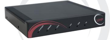
This unique device can even implement multiple access protocols and sophisticated QoS, so that it can work as a fully-fledged TDM/TDMA Hub with one Outbound TDM and up to 4 Inbound TDMA carriers. UHP-200 can switch on-the-fly between the modes, using any of the 8 configuration profiles stored in the device.
