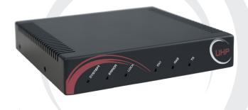
UHP-100 is equipped with two high-speed demodulators together with their independent IF inputs and front ends. The router can simultaneously receive two carriers transmitted via two different satellite beams, which can even be in different frequency bands. The dual demodulator in conjunction with a built-in advanced beam switching algorithm facilitates seamless roaming of mobile satellite terminals between distinct beams of HTS satellites.
